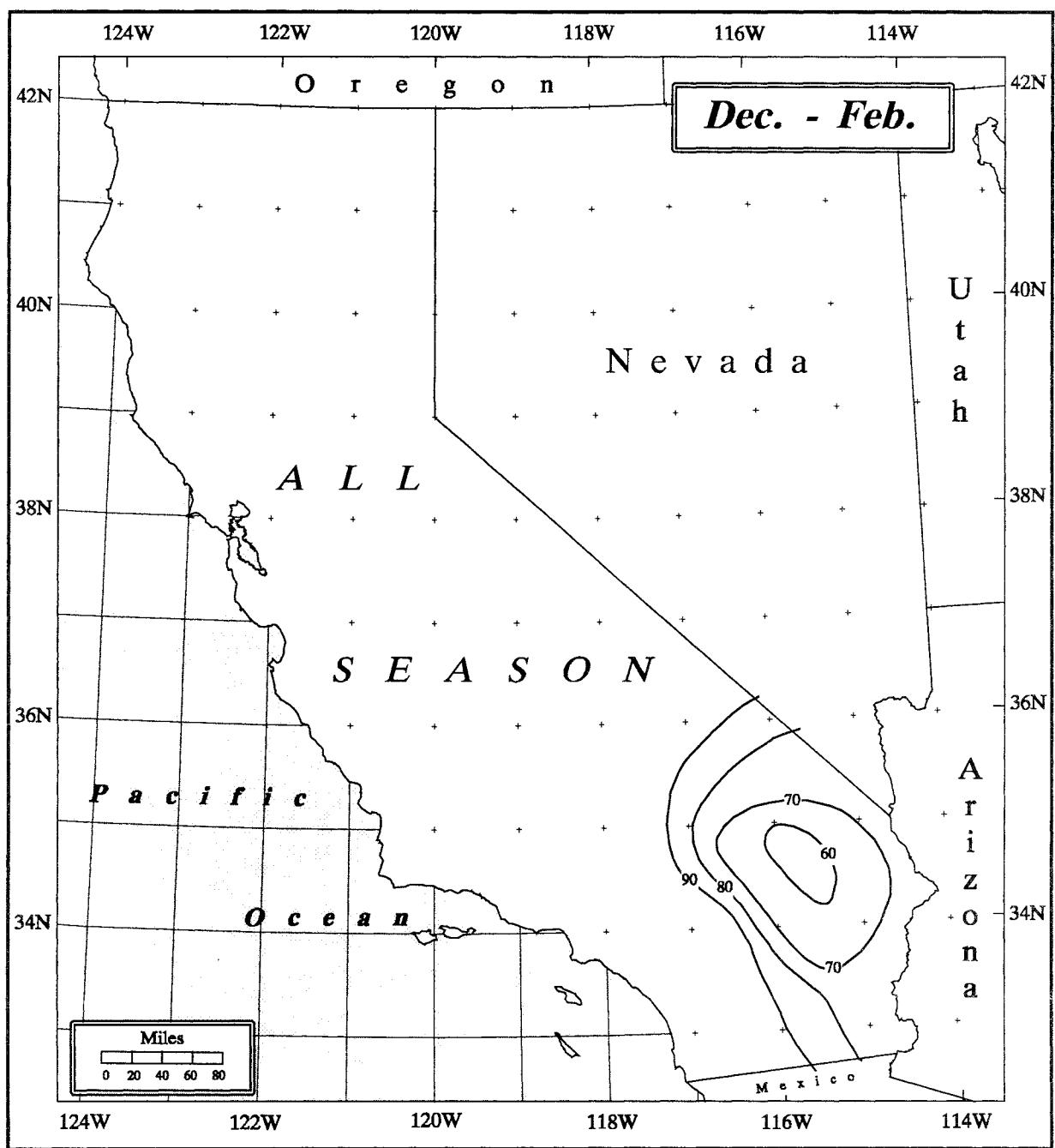
**Figure 2.1.**  $10\text{-mi}^2$  24-hour general-storm PMP for December through February in California as a percent of all-season PMP (Plates 1 and 2).
