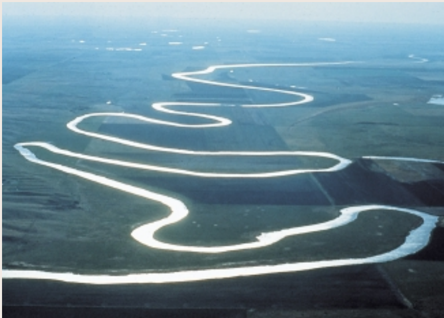
Figure 8.23: The natural meander of a stream. Rivers meander to increase length and reduce gradient. Stream restorations often attempt to reconstruct the channel to a previous meandering condition or one “copied” from a reference reach.
